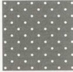
Pattern #457 .052 in. diameter diagonal pattern 21 holes per square inch
