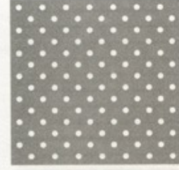
Pattern #914 Mini Perf .052 in. diameter straight line pattern 70 holes per square inch
