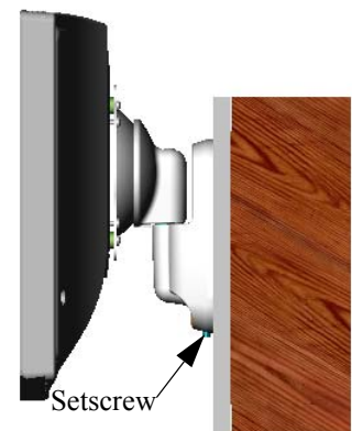
Figure 3. Tighten Setscrew to Secure
