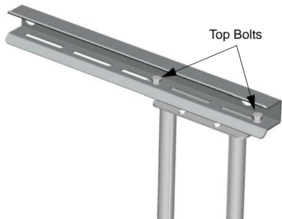
Figure 14. Adjust Swing Arm – Right of Center
