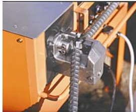
Close up of rebar cutter
