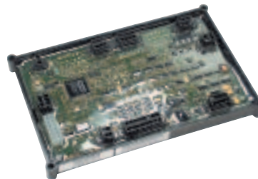
Printed circuit boards are environmentally-shielded using Lincoln's engineered potting and protective frame trays.
