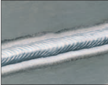
Pulse-On-Pulse™ on 3 mm Aluminum
